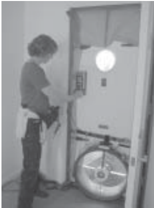
Gail Brownell turns up the fan on the door blower used in house audits. Photo by Dadla Ponzini
